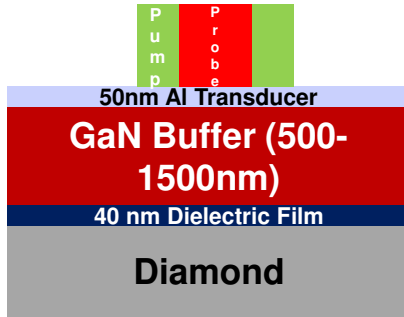
Fig.1 Sample configuration for TDTR measurement of GaN on Diamond TIR
