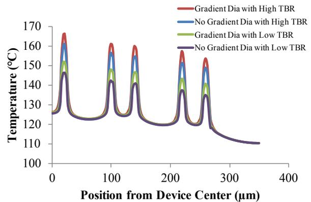
Figure 4. Graph showing the temperature distribution for the channels from the center to the edge of the 10 finger HEMT for all four combinations of TBR and diamond thermal conductivity
