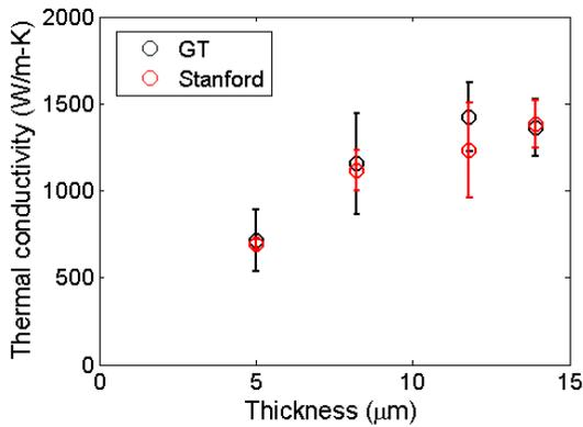
Figure 2. Thermal conductivity plotted versus film thickness, as measured by Stanford and GT, for diamond-on-Si samples.
