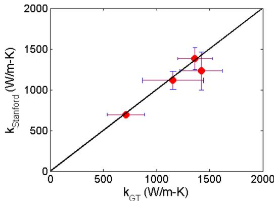
Figure 1. Comparison between thermal conductivities measured by Stanford and GT for 5-13.9  $\mu\text{m}$  diamond-on-Si samples
