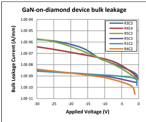
Fig. 2 Leakage measurements for various devices across an older generation GaN-on-diamond wafer.
