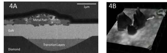
Fig. 4 a) FIB cross-section of device in figure 3a and b) laser confocal microscope image showing post transition etch residue prior to diamond deposition on a separate wafer.
