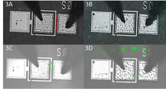
Fig. 3 a) An EMMI image of a high leakage device and b) an EMMI of a low leakage device c) an OBIRCH of the same high leakage device and d) OBIRCH of the same low leakage device.
