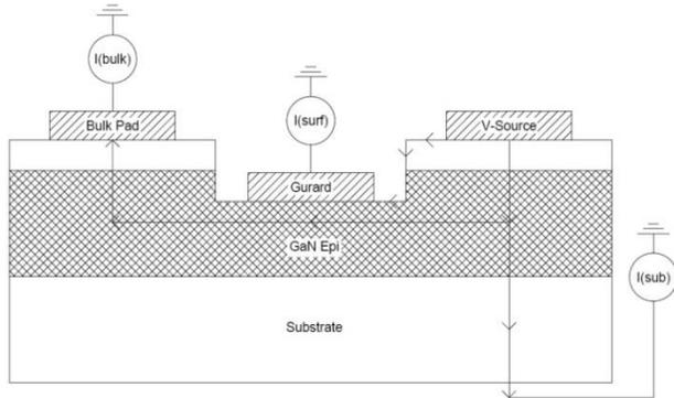
Fig. 1 Test structure used to measure buffer, surface and substrate leakage.
