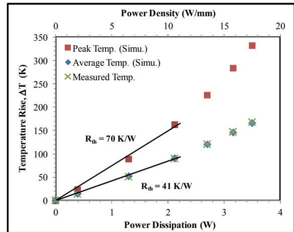
Fig. 7. Temperature rise of a standard 2x100 $\mu\text{m}$  GaN HEMT on SiC with DC power dissipation as measured by micro-Raman and as simulated by fitting the measured data.
