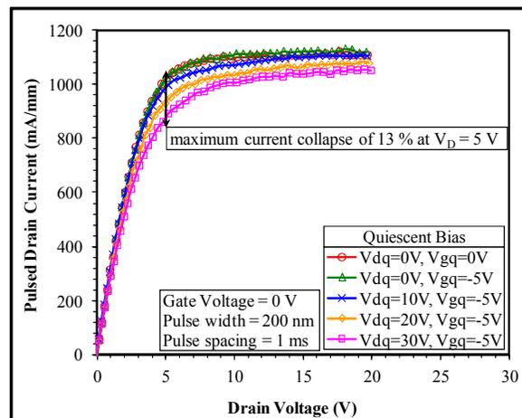
Fig. 3. Pulsed I-V characteristics of a 2x100  $\mu\text{m}$  gate-width GaN HEMT on diamond at various quiescent conditions.
