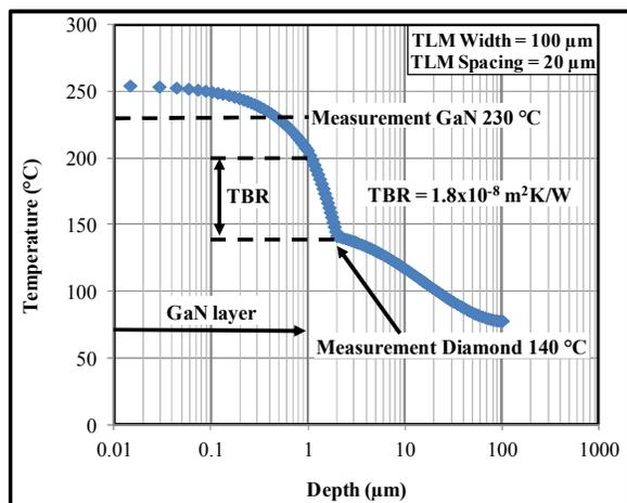
Fig. 8. Depth profile of temperature of a GaN-on-diamond TLM structure using micro-Raman measurements and simulation.
