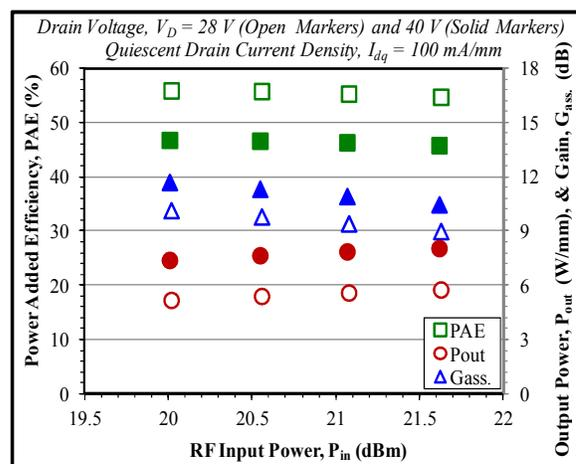
Fig. 4. 10 GHz load pull results of a 2x100  $\mu\text{m}$  GaN HEMT on diamond at different bias conditions.
