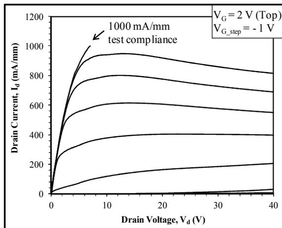
Fig. 2. Drain current characteristics of a 50  $\mu\text{m}$  gate-width GaN HEMT on diamond.
