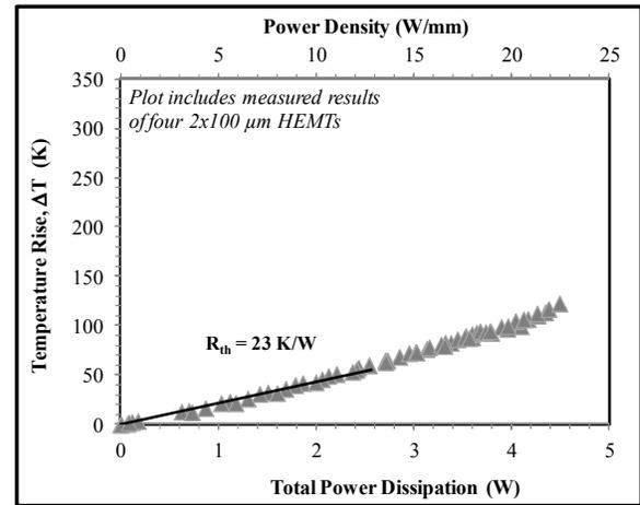
Fig. 5. Temperature rise of 2x100 $\mu\text{m}$  GaN HEMTs on diamond with DC power dissipation measured using an IR camera.
