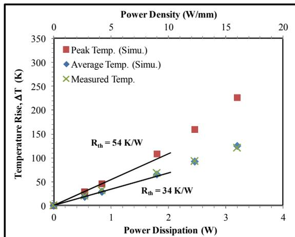
Fig. 6. Temperature rise of a 2x100 $\mu\text{m}$  GaN HEMT on diamond with DC power dissipation as measured by micro-Raman and as simulated by fitting the measured data.
