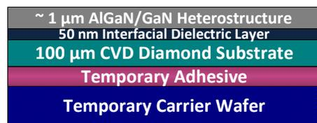
Fig. 1. Schematic cross-section of GaN-on-diamond device wafer mounted on a temporary carrier for processing.
