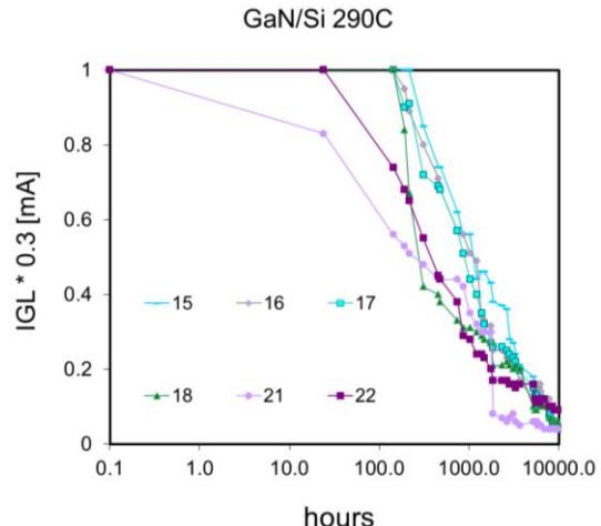
Figure 7 Gate-leakage current measured on 6 GaN-on-Si devices biased with a Source-Drain voltage of 24V. Channel temperature is maintained at 290C.
