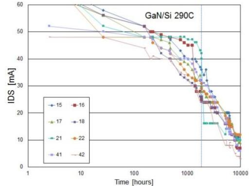
**Figure 5A – GaN-on-Si devices  $I_{DS}$  at  $290^\circ\text{C}$  (phases I+II)**
