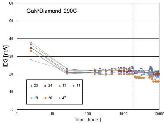
Figure 5B – GaN-on-Diamond devices  $I_{DSS}$  at 290°C (phases I + II).
