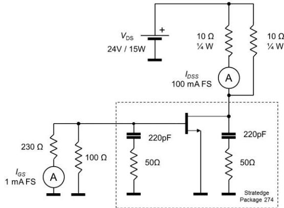
**Figure 3 – Electrical wiring in the life-test system. The gate is at zero bias, connected to ground via ammeter, and the drain is connected to a 24-V power supply. We monitor  $I_{GS}$  (leakage) and  $I_{DS}$  (drain current at zero gate bias).**
