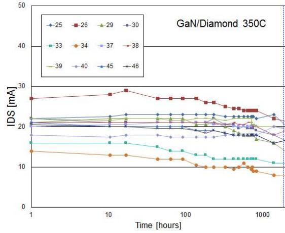
Figure 6B – GaN-on-Diamond devices  $I_{DSS}$  at 350°C (phase II).
