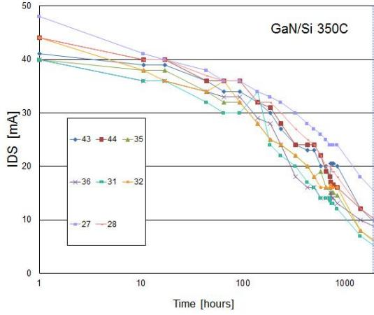
Figure 6A – GaN-on-Si devices  $I_{DSS}$  at 350°C (phase II).
