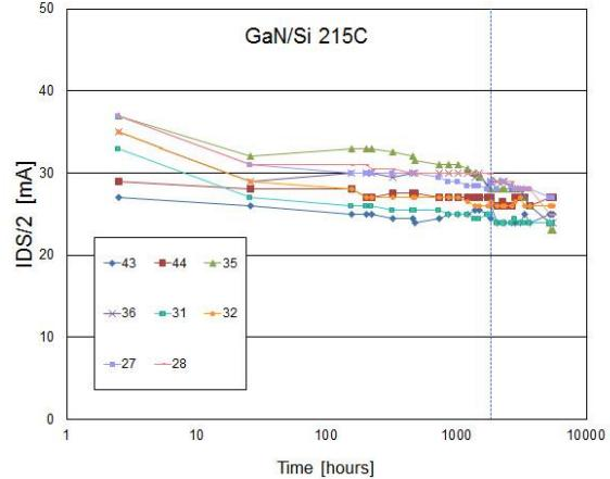
**Figure 4A – GaN-on-Si devices  $I_{DS}$  during first 5,000 hours of life-test at  $215^\circ\text{C}$ .**
