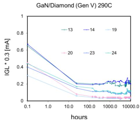
Figure 8 Gate-leakage current measured on 6 GaN-on-Diamond devices biased with a Source-Drain voltage of 24V. Channel temperature is maintained at 290C.
