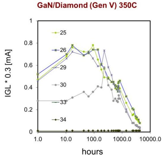
**Figure 10** Gate-leakage current measured on 6 GaN-on-Diamond devices biased with a Source-Drain voltage of 24V. Channel temperature is maintained at 350C.
