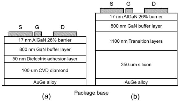
**Figure 1 – Epilayer structure of the GaN-on-Diamond (a) and GaN-on-Si (b) transistors tested.**
