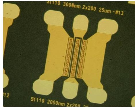
**Figure 2 – Photograph of 2-gate layout of devices used in this experiment.**
