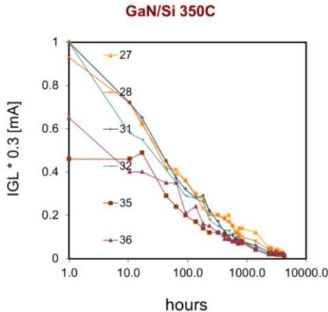
**Figure 9** Gate-leakage current measured on 6 GaN-on-Si devices biased with a Source-Drain voltage of 24V. Channel temperature is maintained at 350C.
