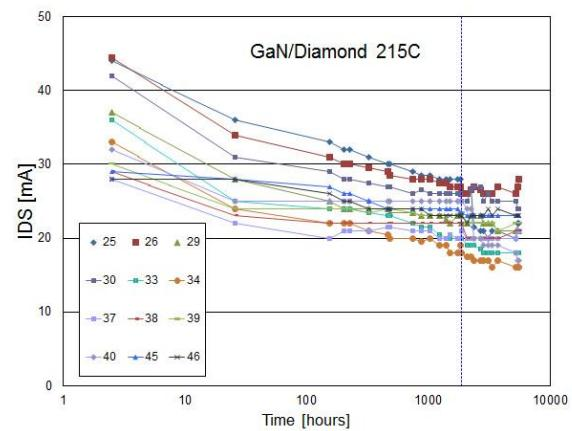
**Figure 4B – GaN-on-Diamond devices  $I_{DS}$  during first 5,000 hours of life-test at  $215^\circ\text{C}$  (phase I).**
